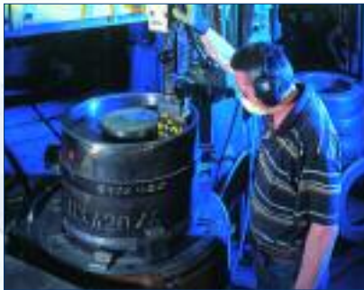
Pressing a grinding wheel to pre-defined instructions
